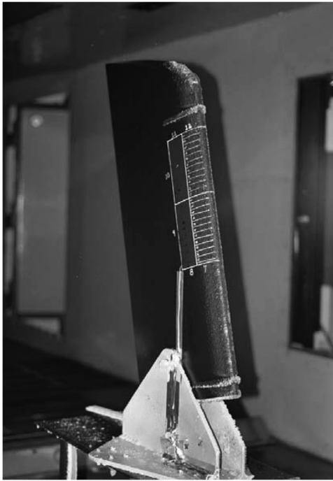
Fig. 9 NACA 0012 swept wing tip in the IRT test section. From Vargas and Reshotko [3,4] (1998).
